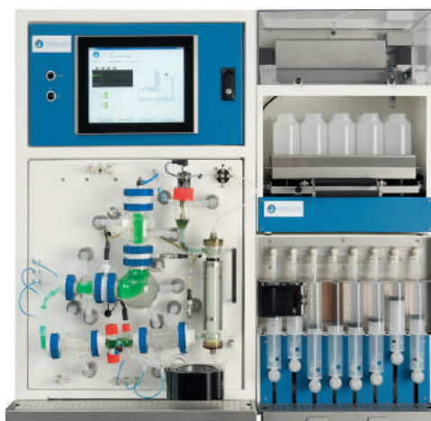
Tiny-TIM system. Model unit (left), sampling unit (top right) and dispensing unit (bottom right).
